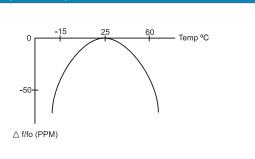
To calculate the frequency stability the parabolic curvature constant (K) is needed. For calculating the stability at 45°C? 1- Change in temperature ( $\Delta$ T) is (45-25) = +20°C 2- Change in frequency is (-0.034 x ( $\Delta$ °C)²) = (-0.035 x (20)² = -13.6ppm
